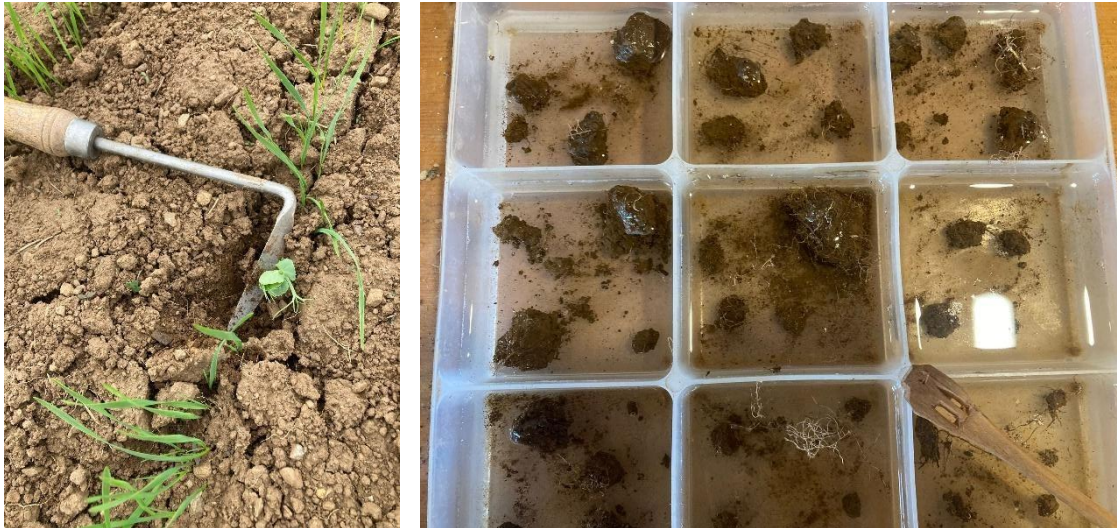
Figure 5 (a) Taking soil aggregate samples from soil adjacent to seedling roots, and one of the trays showing soil aggregate stability after 2 hours of immersion in water.
