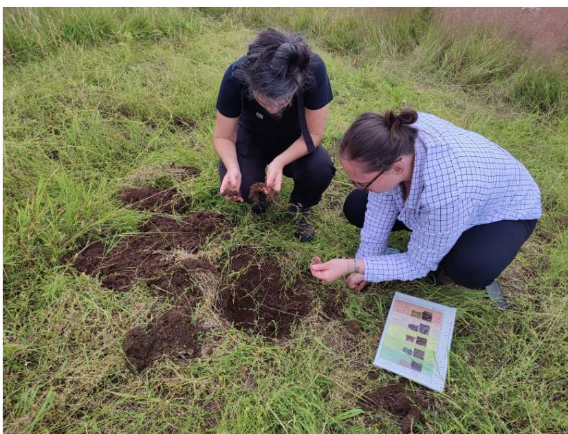
Image 2: Visual Evaluation of Soil Structure (VESS)
