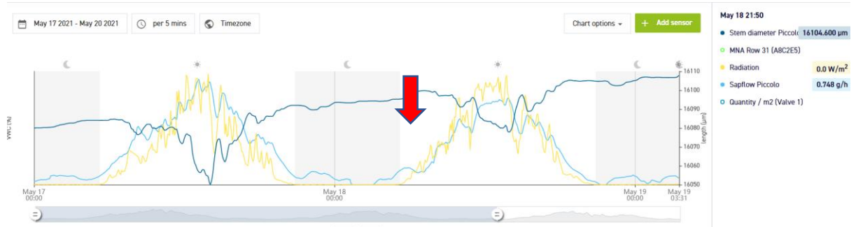
Fig 5 showing lower sap flow with similar radiation.
