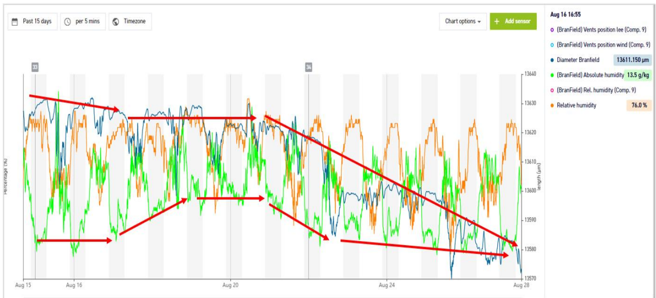
Fig 16 showing longer term effect of reduced humidity
